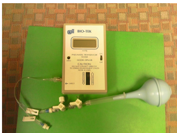
Fig. 1. Equipment used for measuring negative pressures generated by bulb syringes.
