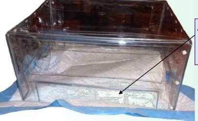
For removal in case of emergencies or other procedures all lines and tubing go under the bottom arches on all 4 sides
